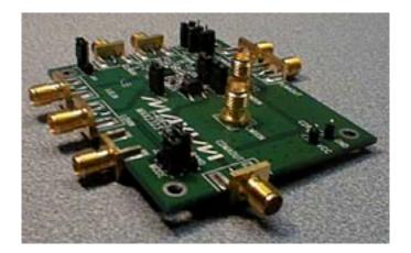
Objective: To apply and measure this dual-band triple-mode CDMA front-end IC in a receiver with all 210MHz IFs.
